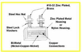
Another major factor to consider is the affect that temperature has on the rating of the circuit protector. As with all thermal devices, as temperatures change the continuous current rating of the circuit protector changes. As stated earlier, all Pollak circuit protectors are designed to run continuously at 100% or rated current at 77°F. The bottom chart shows the effect temperature has on the rated current for circuit protectors.
